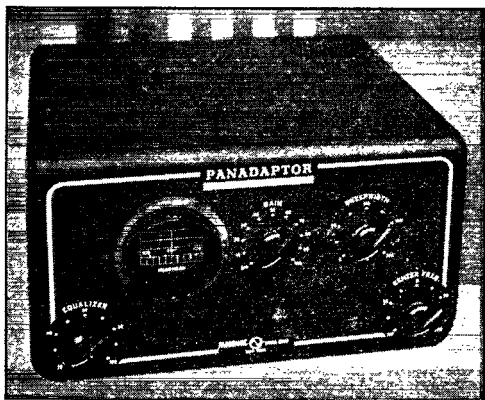
A panel view of the modern panoramic adaptor. The "equalizer" control at the lower left-hand corner allows compensation for the variation in receiver front-end selectivity on the various bands.
