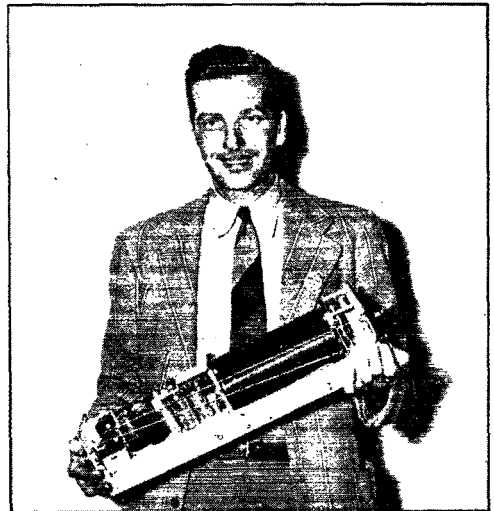
Phil Gildersleeve, W1CJD, city editor of the Middletown Press and famous QST cartoonist, holds one of the 2-inch Vericon cameras during a recent demonstration of the equipment to the press. The cord stretched along the unit is part of the automatic iris control system.
