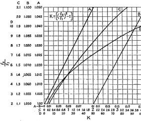
Fig. 2 — Chart for determining K from the ratio  $f_2f_1$ .
