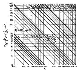
Fig. 3 — Chart for evaluating  $C_{t_1}$  from selected values of  $C_1$  and K.
