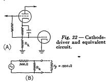
point  $Q_1$  we draw a load line for 8000 ohms — 8000 ohms because the 6 volts across  $R_1$  is held constant by the by-pass condenser across it.
