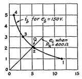
Fig. 18 — Graph for finding zero-signal bias for pentode with resistance load.
