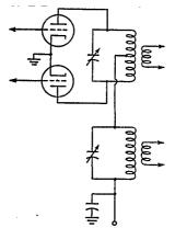
Fig. 2 — Output circuit for coupling both parallel and push-pull components.
