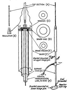
Fig. 1 — Sketch showing details of construction of the 112-Mc. coaxial antenna.
