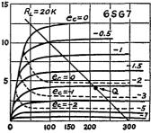
Fig. 17 — 20,000-ohm load line plotted on 6SG7 characteristics.
