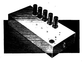
Last month we hinted about new gadgets for the amateur as soon as the war is won. Here is one such unit which we are sure the gang will appreciate—a CASCADE FREQUENCY MULTIPLIER designed to produce optimum output over the whole band from 160 to 10 meters without retuning. Band selection is accomplished by a remote push button and output frequency is controlled by any good ECO.
