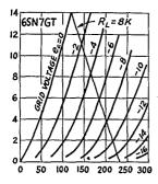
Fig. 21 — 6SN7 characteristics (one triode unit).
