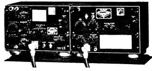
HERE ARE A FEW of many types of the Navy's small craft which maintain communication with this Collins designed TCS radio transmitter and receiver combination. This equipment is so sturdy, handy and reliable, and packs so much power and sensitivity into so little space, that it finds numerous Naval applications ashore as well as afloat. Usually the
