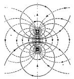
changing electric field can create a magnetic field. Now carry the process one step further, as shown in Fig. 4. The electric field here is seen to set up a new magnetic field in the surrounding dielectric — circling around the displacement current, which varies according to the non-linearity of the initial field. Note that the new induced field is entirely disassociated from any conductor; it exists wholly in the dielectric.
