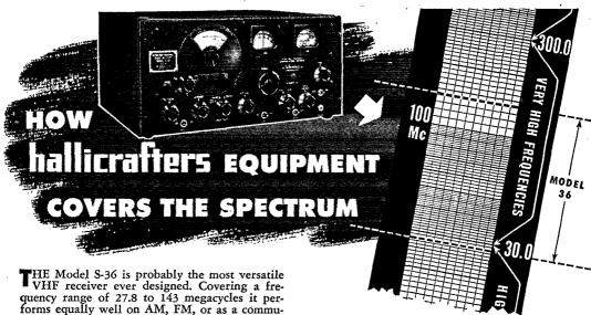
THE Model S-36 is probably the most versatile VHF receiver ever designed. Covering a frequency range of 27.8 to 143 megacycles it performs equally well on AM, FM, or as a communications receiver for CW telegraphy. Equipment of this type was introduced by Hallicrafters more than five years ago and clearly anticipated the present trend toward improved service on the higher frequencies.
