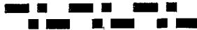
Fig. 3 — Graphic representation of the overlapping of the "A" and "N" signals to form a continuous steady signal along the range course bearing.
