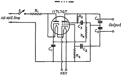
Fig. 2 — Circuit diagram of simple code-practice oscillator.
