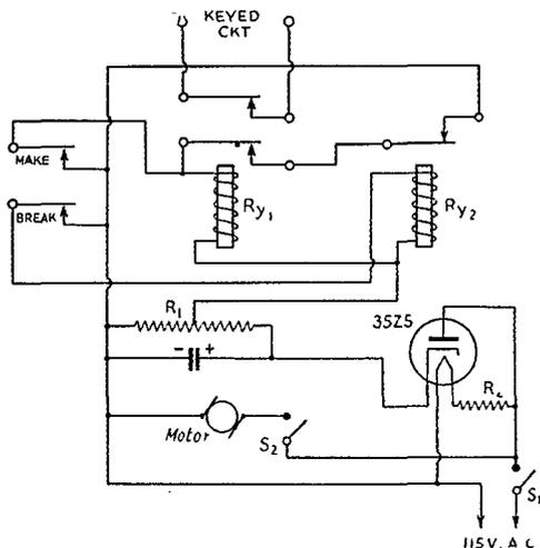
Fig. 2 — Circuit diagram of the code reproducer. C — 40- $\mu$ fd. electrolytic, 150 volts. (Smaller capacities will do.) R<sub>1</sub> — 6000-ohm bleeder, tapped to give about 40 volts for the relays used. R<sub>2</sub> — Heater dropping resistor, 500 to 550 ohms. Ry<sub>1</sub>, Ry<sub>2</sub> — See text. S<sub>1</sub>, S<sub>2</sub> — S.p.s.t. toggle.
