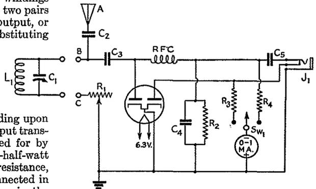
Fig. 3 — Circuit diagram of the modulation indicator.
