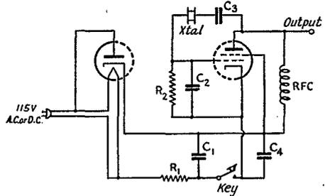
Fig. 1 — Simple circuit for crystal testing employing a 117L7GT.
