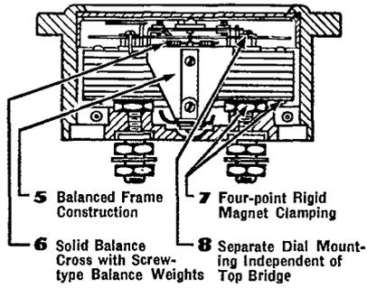
Thin-Line Instruments also have Standard Large Coil Triplet Movements. Furnished with Osmium pivots for special requirements. All these features make for greater rigidity under vibration; greater permanence of calibration; greater user satisfaction.
