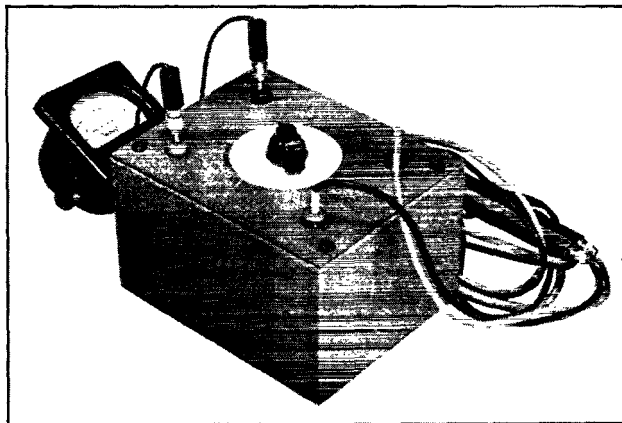
A photograph of the multi-range volt-milliammeter. The leads of an internal 0-1 ma. meter are plugged into the jacks at the top of the box. Test leads plug into the jacks at the bottom.
