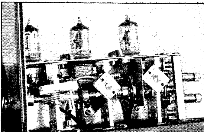
Inside the converter unit, showing the arrangement of tuning condensers. The layout is quite compact, every effort having been made to keep leads as short as possible.
