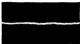
Oscillogram showing noiseless performance of Bradleyunit Resistors.
