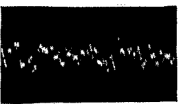
Oscillogram showing noisy performance of other types of resistors
