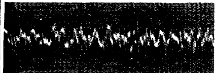
Oscillogram showing noisy performance of other types of resistors.
