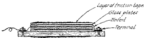
How the glass plate fixed condensers are put together (The right number of plates is not shown)
