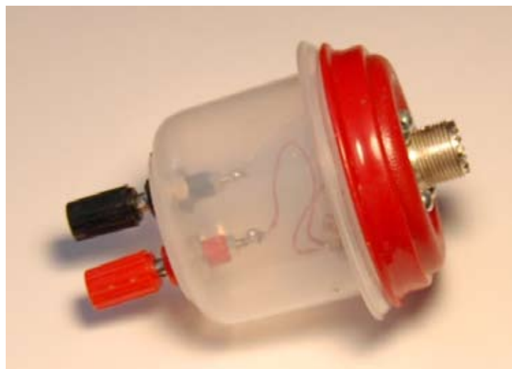
RF matching transformer in a weather-tight plastic food storage container.
