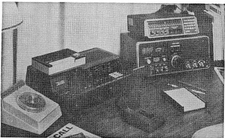
Fig. 9-1. A dream shack communications post based on equipment from Radio Shack. It includes a 40-channel SSB/AM rig for CB, a Weatheradio alert receiver, a VHF/UHF programmable scanner, and a DX-300 receiver that covers from 10 kHz to 30 MHz.
