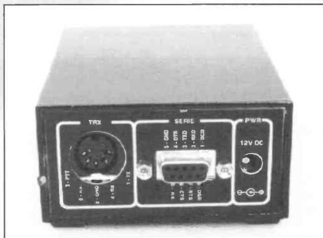
The radio connector on the rear panel follows the TAPR standard, optional ready-wired leads are readily available
