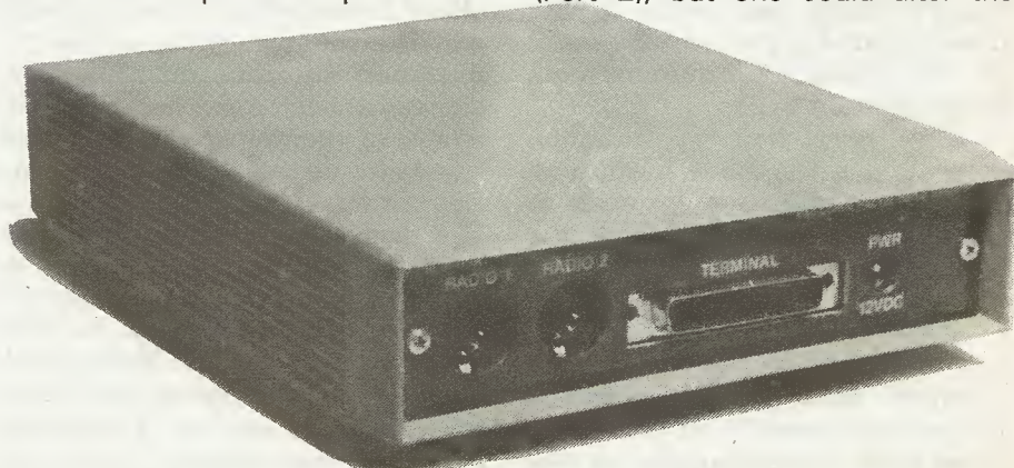
Rear panel connections showing the separate HF and VHF input/output sockets
