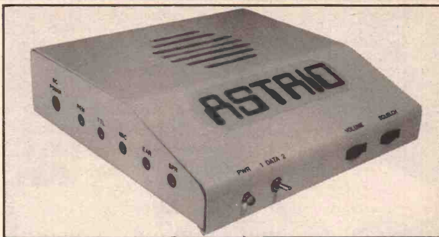
A white box solution to the problem of receiving UOSAT data on your home micro.
