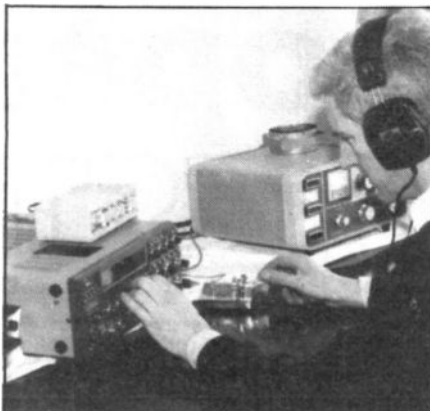
Broadband 'solid state' transceivers, like the TS930S used at GJ3SXW, are becoming universal for multiband contests, with their 'no-tune' band change ability.
