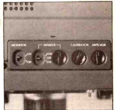
The calibrator, 'monitor' and VOX controls are located on a small panel on top of the '745 just behind the fascia.
