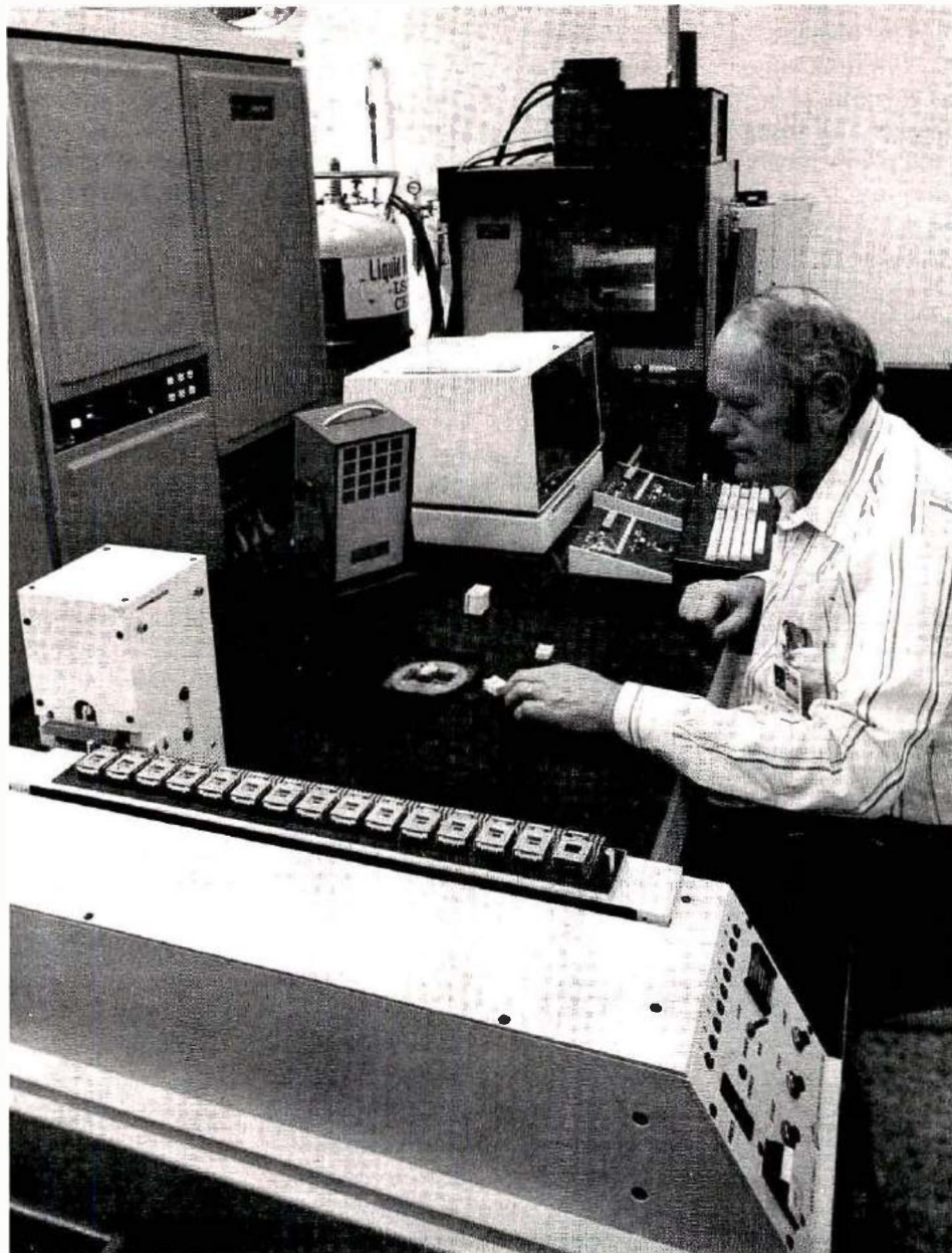
Digital integrated circuits require complex test equipment. Shown here is a Fairchild Sentry 7 in use at Raytheon Corp. The large desk contains digital driver/detectors for each pin of the IC package. A tester such as this costs $500,000.
