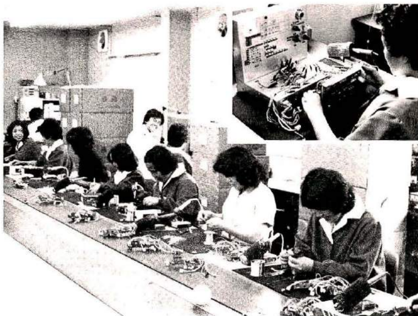
Quick and nimble fingers wiring up sub-assemblies on a production line at the ICOM factory. Inset: Some of the test gear is homebrewed, like this one designed to test front-panel wiring on the IC-701 transceivers. The rubber elastic strap around the edge of the panel protects it from scratches.
