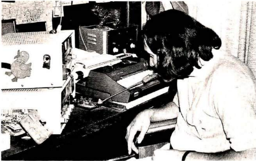
Larry forms Morse code by pressing the rubber-tipped stick to the key, and moving his head up and down.
