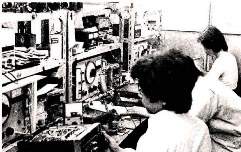
ICOM vhf gear on the test bench, receiving the standard checks applied to every piece after assembly.
