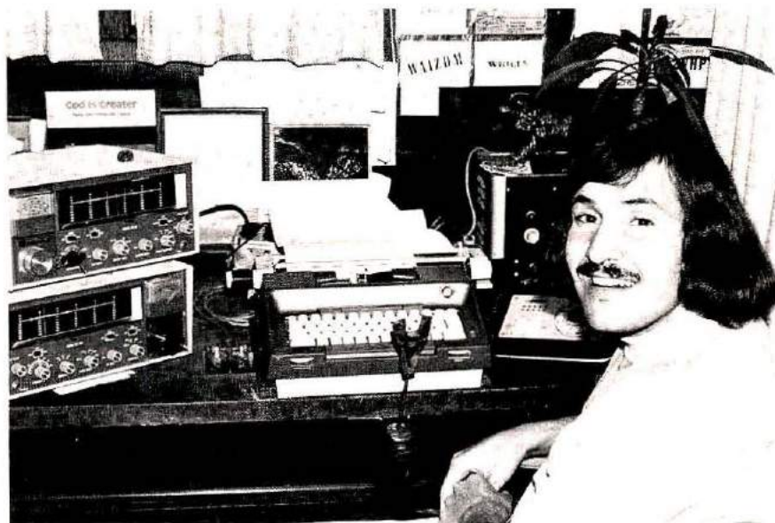
Larry, WB3IGT, at his ham station. The equipment, at left, is a Hallicrafters transmitter and receiver. The forked device in front of the typewriter is Larry's contact with the Amateur world.
