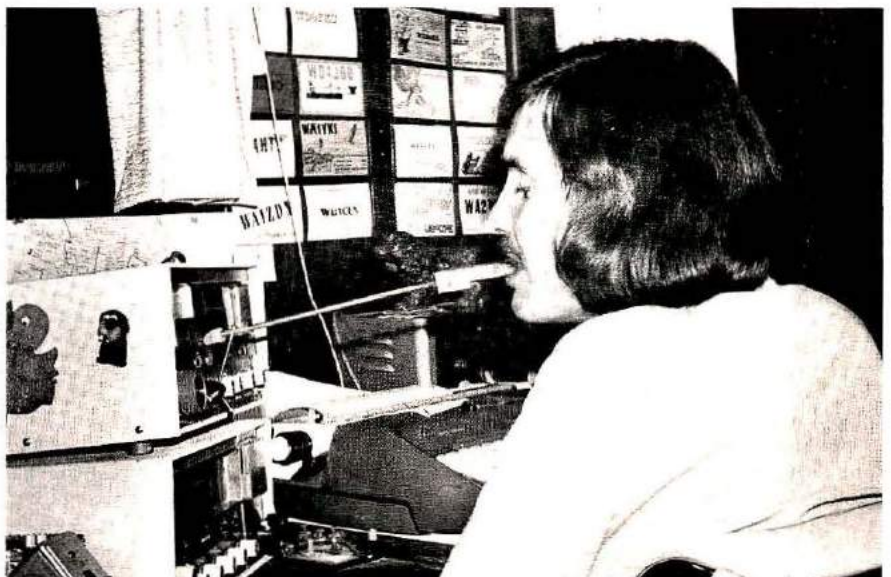
Tuning is accomplished by using the stick to press against long screws in the control knobs. Larry's next project is to get his General-class ticket; then, he can use voice-operated transmit systems (VOX).
