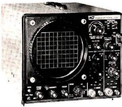
Fig. 6 An auxiliary or "out-board" device that can be attached to an oscilloscope for the purpose of analyzing circuit components such as semiconductors, resistors, capacitors; and shorted or open circuits.
