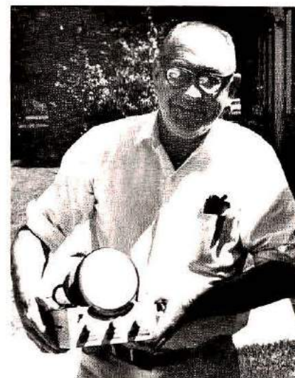
Dexter Phibbs, W4IPA, looks very proud of his homebrew monitor. It is compact and rugged, with a P-7 phosphor screen. The power supply is separate.
