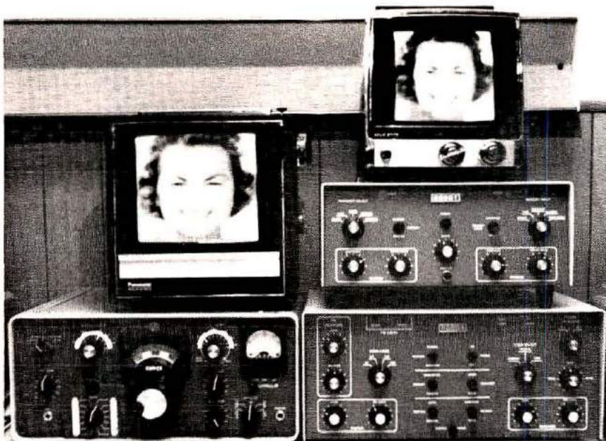
Fig. 8. Double-decker scan conversion in W2DD's shack. The pyramid at the right includes a Robot model 300 scan converter on the bottom, a Robot model 400 Digital scan converter in the middle, and a Sony TV set on top.
