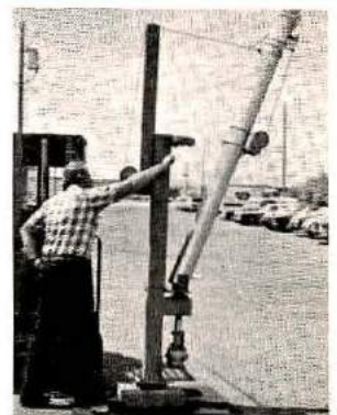
Tilting the tower over is a one-man task with the Wilson bases. (Shown above is the RB-61A.)
