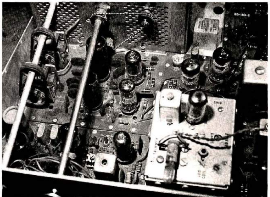
Fig. 2. The first thing is to inspect the chassis against the service manual and make a list of missing or broken parts such as switches, insulators, or electronic parts. Check each component thoroughly. Use a magnifying glass to look for small components. Probe around the wiring with a pencil to ferret out missing or broken components.
