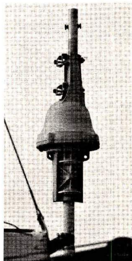
If your finish-line boat is anchored to prevent swinging, you can use a rotator and small beam antenna for improved communications with the yacht-club station.
