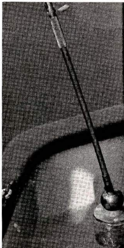
A mobile ball mount provides a versatile system of fastening the whip assembly at a convenient location. You can angle the whip to keep it away from swinging booms.
