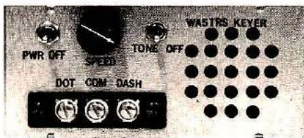
Simple electronic keyer has speed range from 4 to 26 words per minute and has a built-in sidetone monitor.
