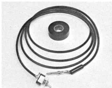
fig. 10. Remote-keying unit for use while testing antennas.
