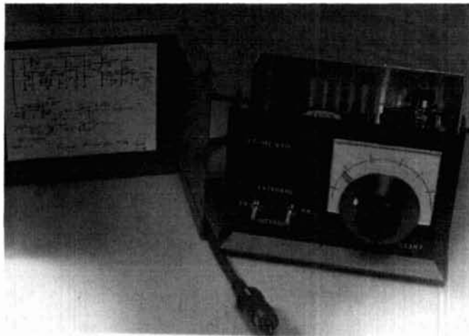
Front view of the VFO with the cover removed showing the DIN plug and the circuit diagram inside the lid.
