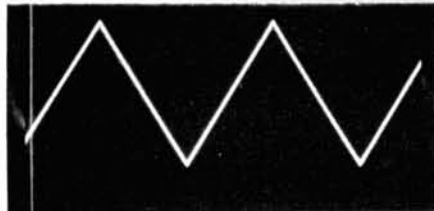
Triangle waveform at a frequency of one-half of the sawtooth output.
