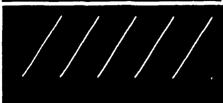
The "normal" output of the sawtooth generator.
