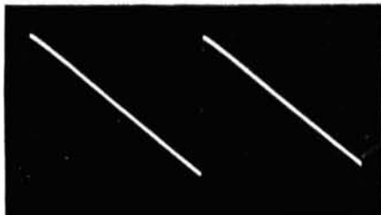
Negative-going (inverted) sawtooth waveform.
