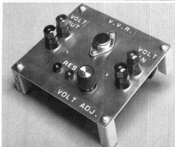
Top view of VVR showing ceramic standoffs.
