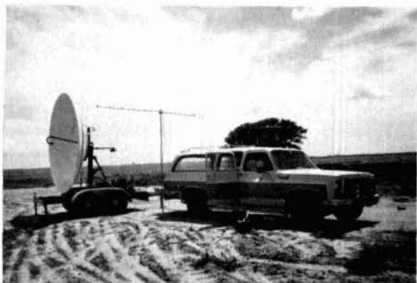
One of the participants in the new 5760-MHz DX records was WA5ICW using his 10-foot "portable" dish setup near Moses, New Mexico.
