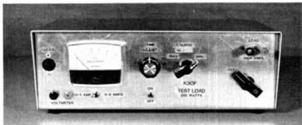
The multi-tapped resistor is the heart of the test load. Note the heavy-duty switch at the upper right for high amps.
