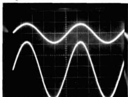
Input (top) and output (bottom) waveforms of gain of +2 noninverting follower.
