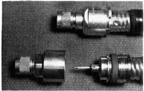
fig. 3. Partially and fully assembled connectors are pictured on 7/8" hardline coax.
