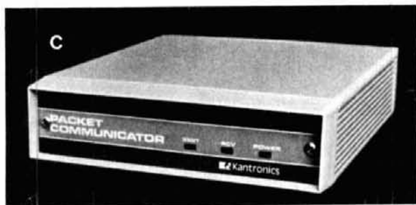
fig. 2B. Packet terminal units from (A) AEA, (B) Heathkit, and (C) Kantronics.
