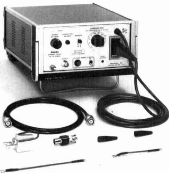
fig. 12A. The P6042 current probe and accessories.
