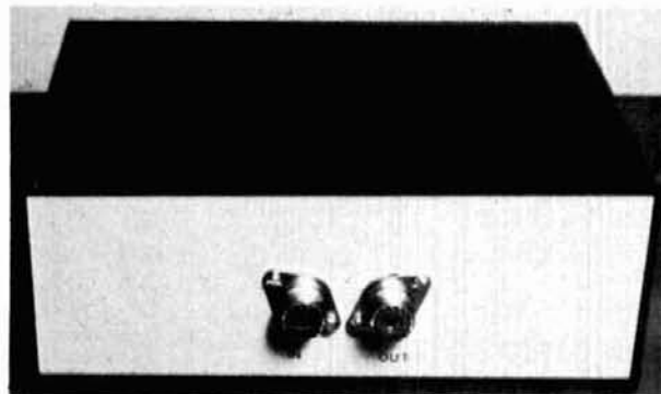
Front and rear views of the completed wattmeter. Lettering is rub-on type; striping is 1/16-inch PC layout tape.
