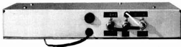
Rear panel of heterodyne scaler showing L.O. changing jacks.
