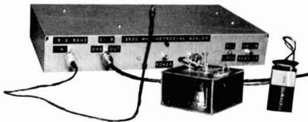
Close-up of scaler, scaler pickup antenna, and a microwave oscillator under test. Note polarization of oscillator.
