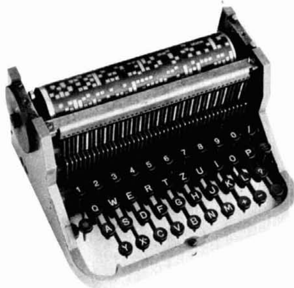
Transmitter section of the original Hellschreiber. The coded drum turns one revolution per character. Every time a key is pressed, one turn of the drum produces a series of pulses by the contact with one series of lamellas.
