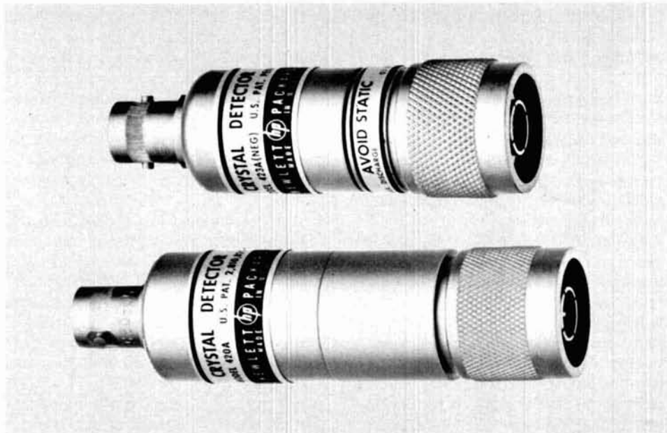
The Hewlett-Packard models 420A and 423A Crystal Detectors are typical of the many detectors which can be used with the swr indicator. Both detectors are usable from 10 MHz to 12.4 GHz. The response of the 420A, on the top, is \pm 3.5 dB with a maximum vswr of 3.0. The 423A is flat within \pm 0.5 dB and has a maximum vswr of 1.5 (1.2 below 4.5 GHz). (Photo courtesy of Hewlett-Packard Company)
