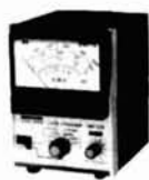
LPM-885 SWR Watt Meter A sensitive, in-line type power meter which measures SWR of x mission lines and power output from 1.8 to 54MHz. Facilitates adjustment of x'mitter and antenna systems for better results. May be left in circuit for continuous power output monitoring in the 1-1000W range. SWR Power Detector circuit assembly separates for remote measurements. Forward-to Reverse power ratio is used for accurate SWR readings. $99.95
