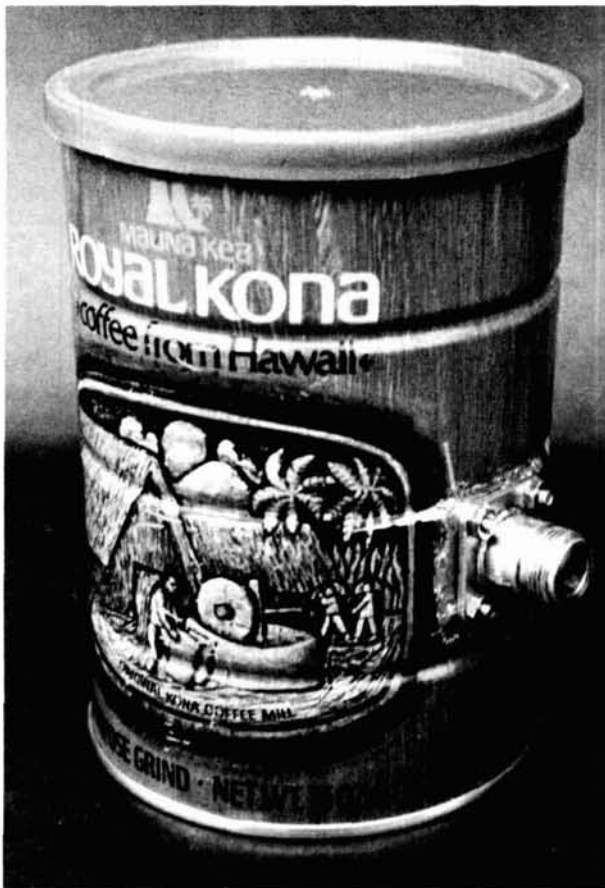
Plastic coffee-can lid makes an effective rf-transparent radome that's bird and weatherproof.
