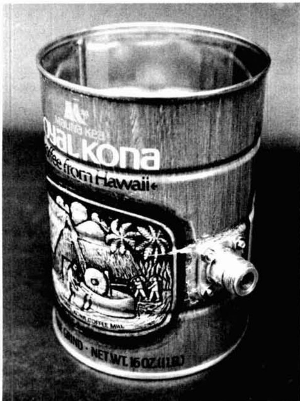
Unpainted feed horn made from a 1-pound (.45kg) coffee can
