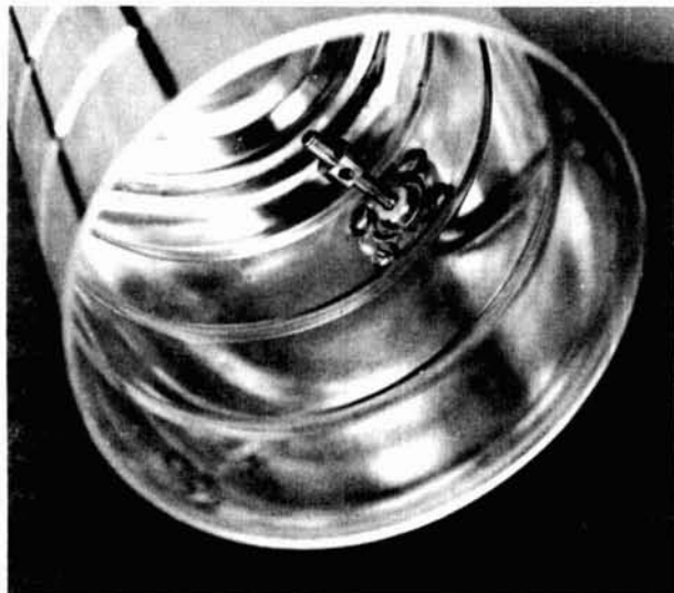
Inside view of unpainted horn showing rf-probe installation.
