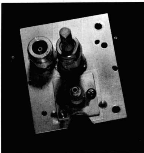
Exterior view of the cathode partition.
