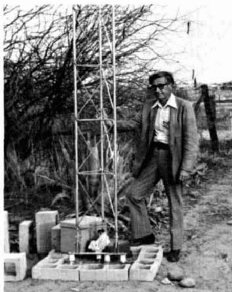
Author W7IV supporting W7IR's antenna. Concrete base is 18 inches (45.7cm) by 1 foot (30.5cm). Tuning network and ceramic insulators are shown.
