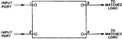
fig. 1. Block diagram of hybrid coupler. This device divides power between two matched loads.
