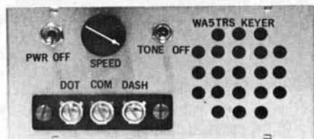
Simple electronic keyer has speed range from 4 to 26 words per minute and has built-in sidetone monitor.
