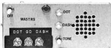
Variable dot- and dash-length keyer has built-in sidetone monitor. Variable controls in center of front panel control dot and dash length.
