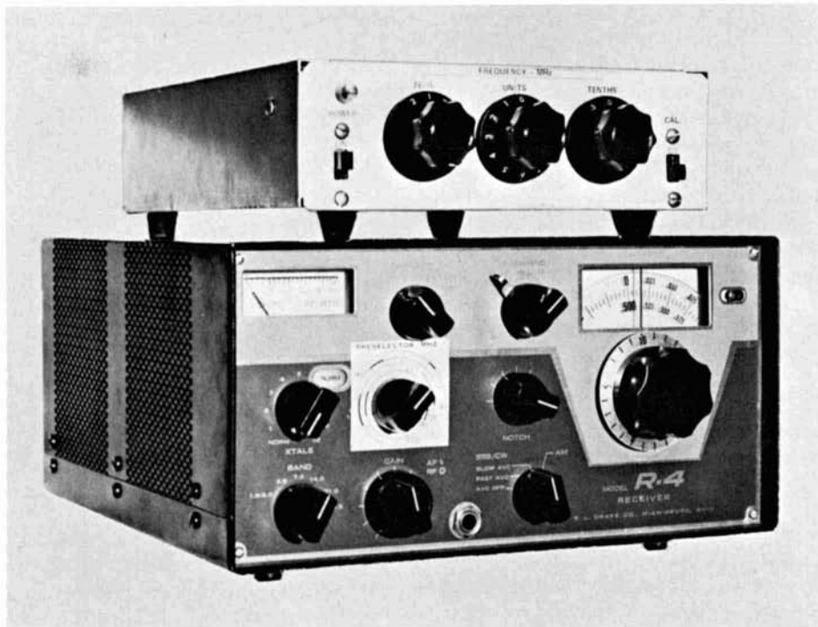
The frequency synthesizer atop the Drake R-4 receiver, which has the new general-coverage preselector scale on its front panel. Operating the equipment in this physical configuration is not recommended because the synthesizer interferes with convection flow from the R-4.
