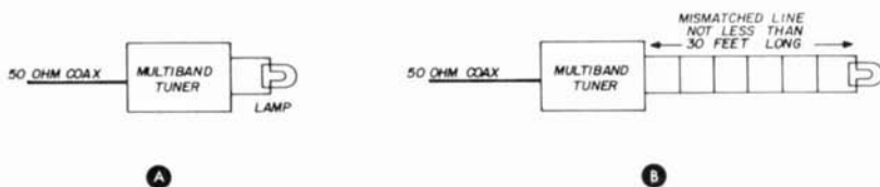
fig. 5. Test circuits. "Compatible" tuner, A , will show same lamp brilliance on all bands. An "incompatible" tuner, with feed line connected as in B , will not deliver full power to the lamp on some bands.
