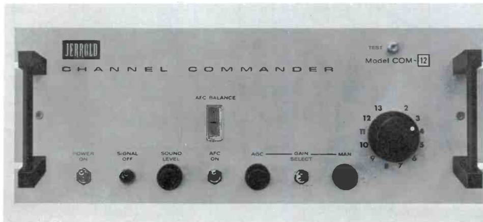
The new single channel, head end unit for the 12 channel system
