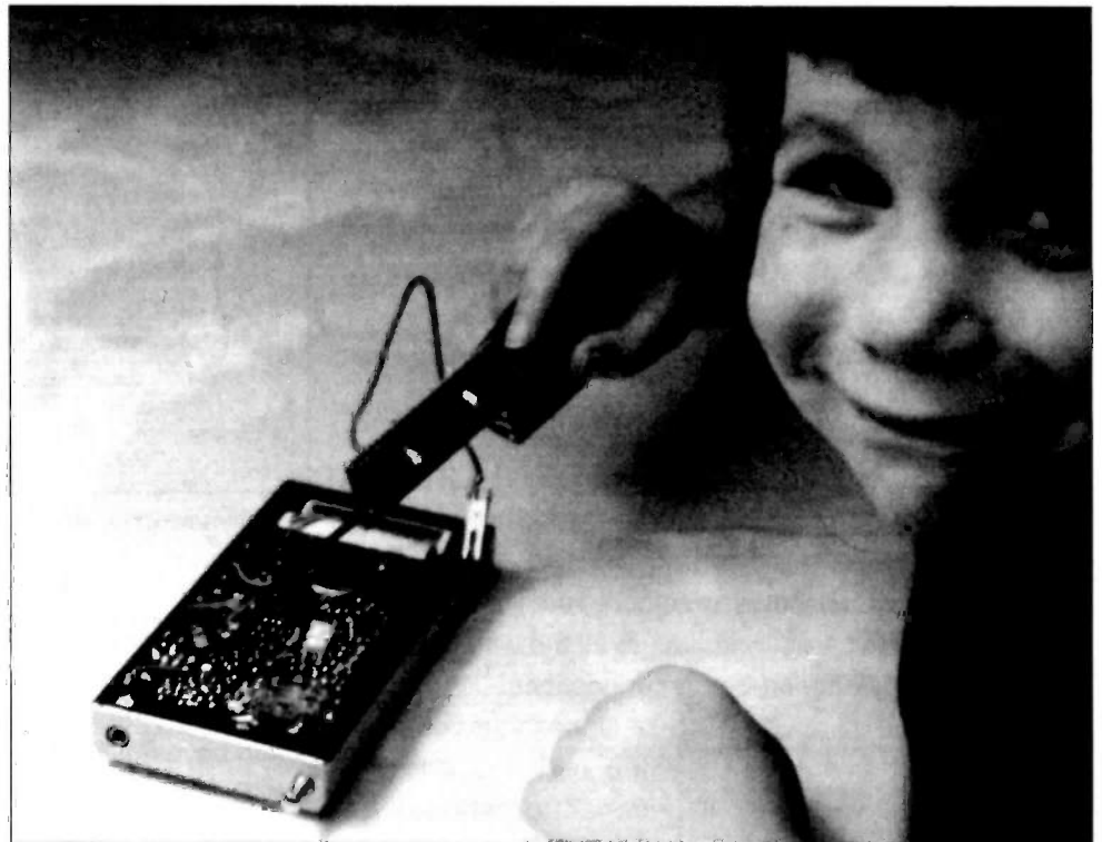
Signal injector being used to test a transistor
