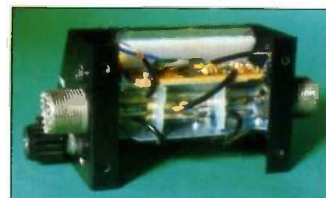
Inside an SWR meter showing a metal trough line.
