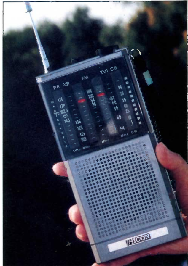
The pre-amplifier gives improved sensitivity to this air-band radio.
