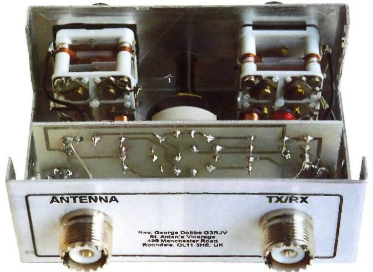
Rear of the ATU-1, showing input and output connectors, the printed circuit board with switch and the two variable capacitors, C1 and C2.
