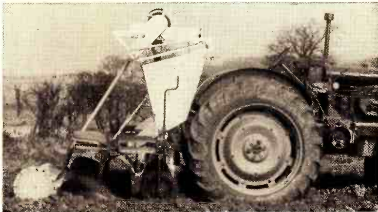
The advantage of placing fertiliser in bands close to the seed has been clearly demonstrated: this fertiliser-placement equipment was designed by the institute
