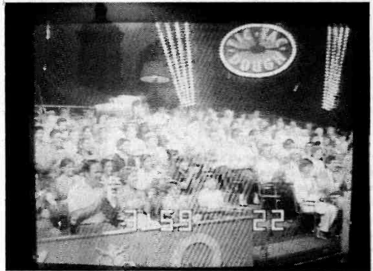
Picture 12 shows the same problem. In this instance the source was channel 3 signal from a VCR RF output feeding back into the cable causing interference to channel 4.
