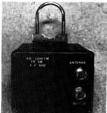
23 CM Preamp with T/R switching
