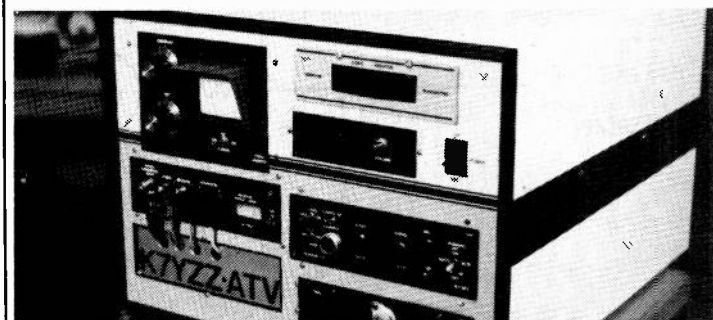
434MHZ in 923MHz out 40 W ATV Repeater on air for Western Washington Amateur Television Society, Jan. 6, 1990. The MKII Model built by "Mr. Wizzard" K7YZZ.
