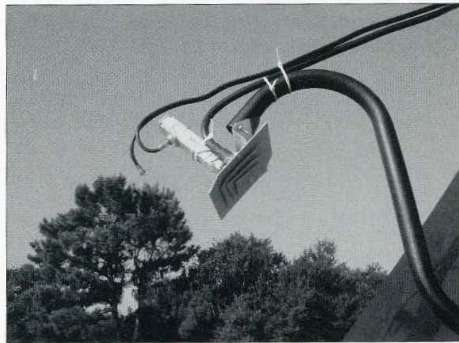
Photo B. An elegant dual-band, circular-patch feed system provides L-band uplink and S-band downlink for AO-40 operation during Field Day 2003 at K5OE. (K5OE photo)
