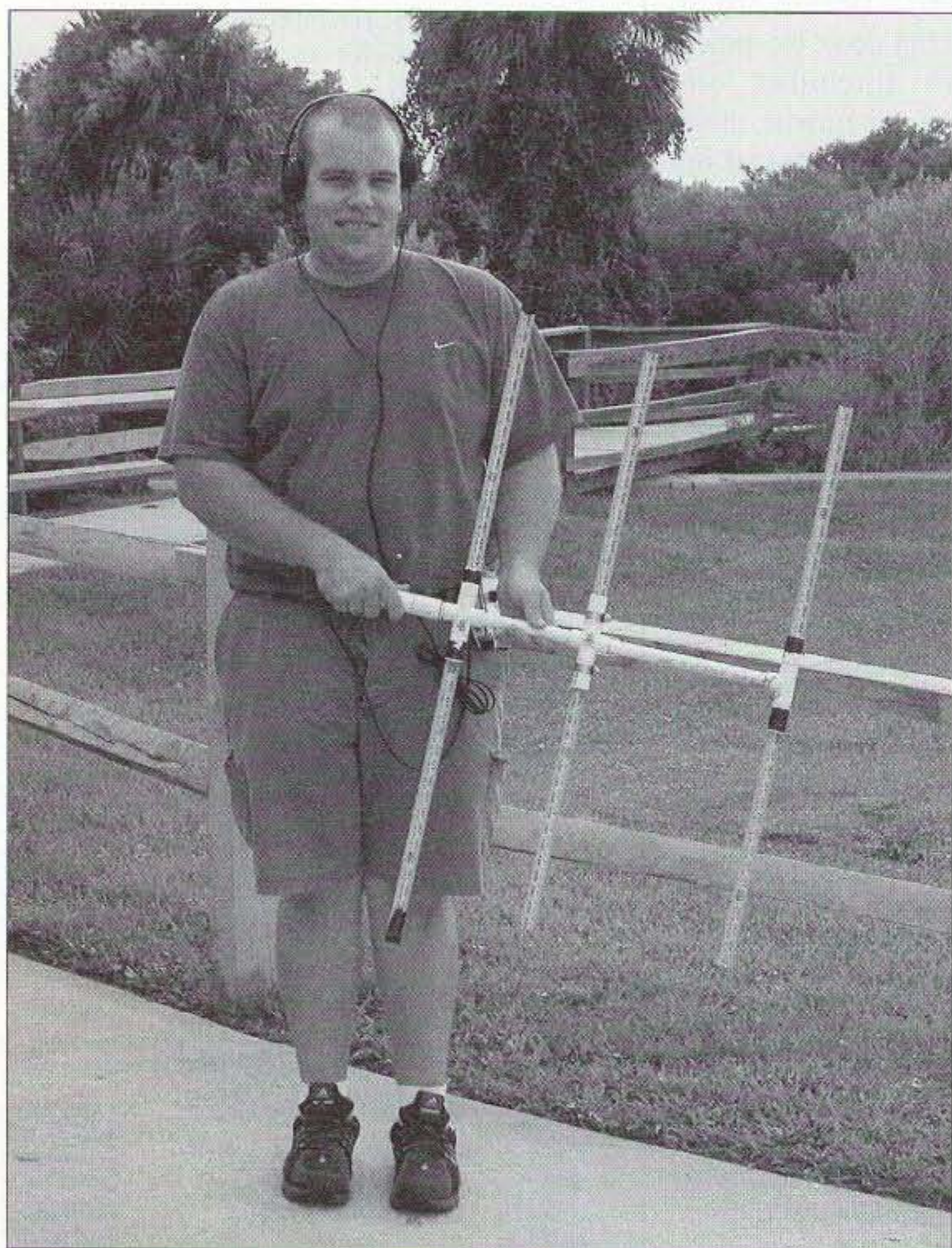
Photo A. Tim Van Nes N9EL won the first Daytona ARDF event using a steel-tape yagi for two-meter foxhunting. Plans for this antenna are on the Web. (All photos by John Munsey KB3GK)
