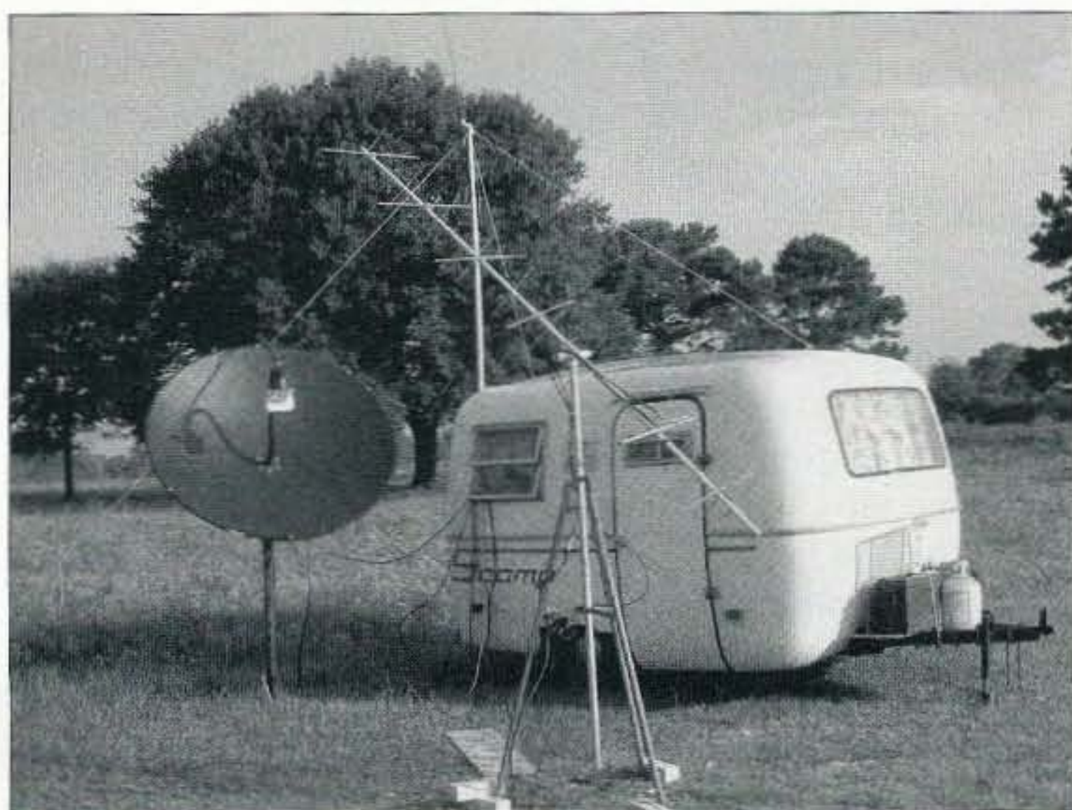
Photo A. A five-foot dish, dual-band yagi, 10-meter vertical, and a Scamp do it all for K5OE and AG5RS during Field Day 2003. (K5OE photo)
