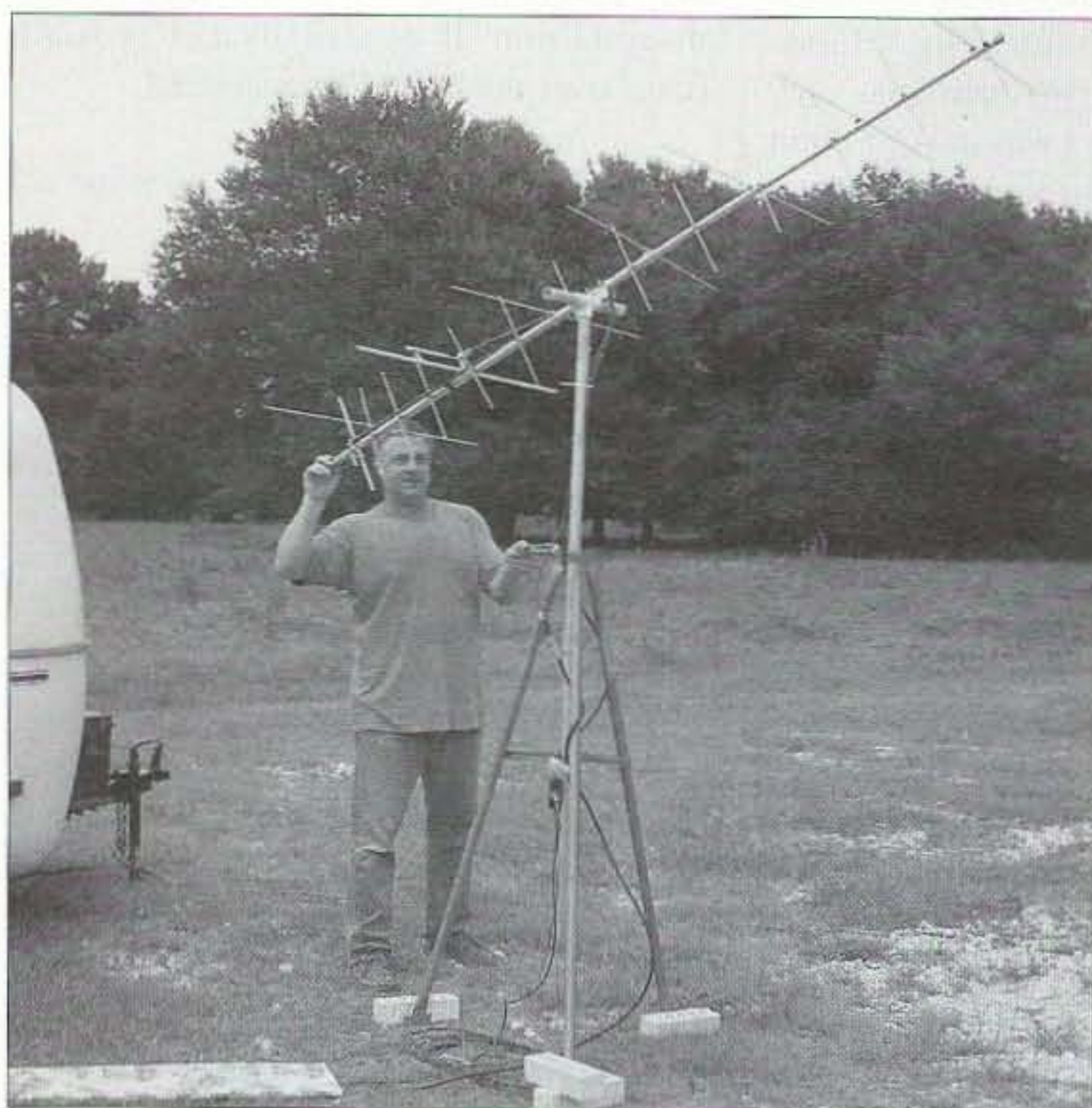
Photo D. Ron AG5RS demonstrates the high-tech rotator system on the dual-band yagi (2 meters and 70 cm) during Field Day 2003. (K5OE photo)
