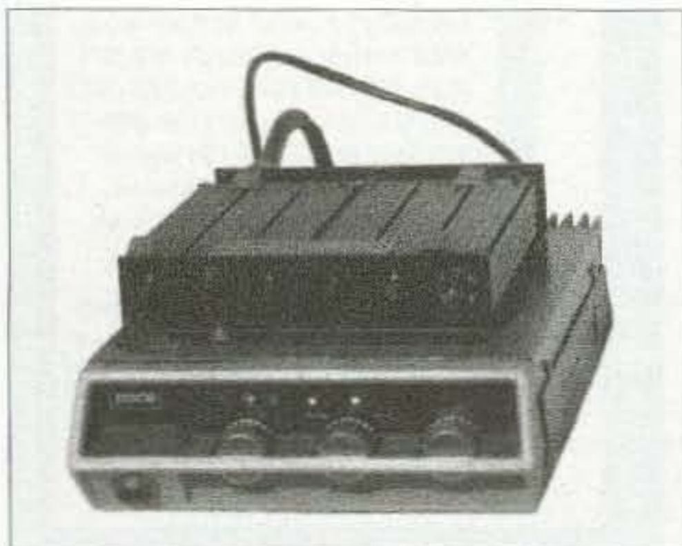
Photo A. This is a picture of the completed portable repeater. A Telemobile Duplexer is mounted to the radio, allowing it to operate with one antenna.
