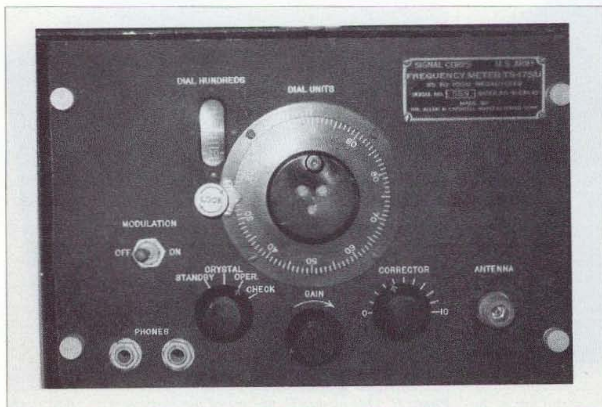
Photo K. Frequency meter dials provided the greatest accuracy and setting repeatability of any dial during the 1940-1950 era.
