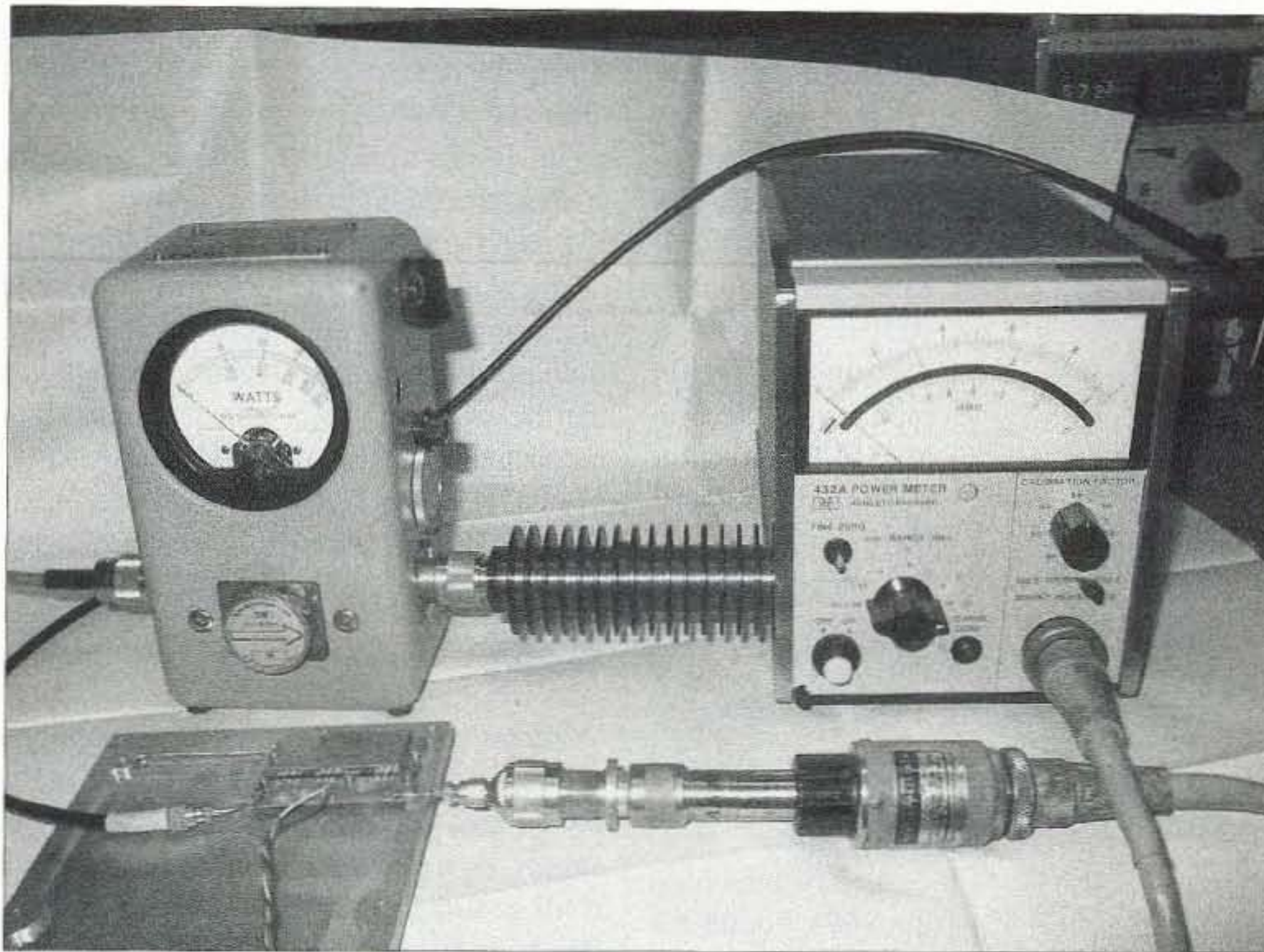
Photo B. Test bench devices used for testing the amplifier include RF sweeper (not shown) for RF drive. For measurements I use both a Bird 43 power meter for coarse work and a HP432 power meter for more exact results. I like to use the Bird 43 RF power measurements and the HP432 and suitable attenuators to do the final exacting measurements.
