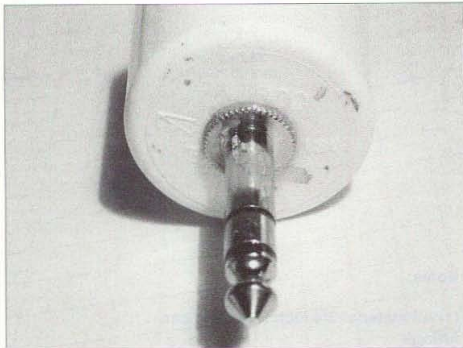
Photo J. 3-circuit phone plug mounted in pipe cap.
