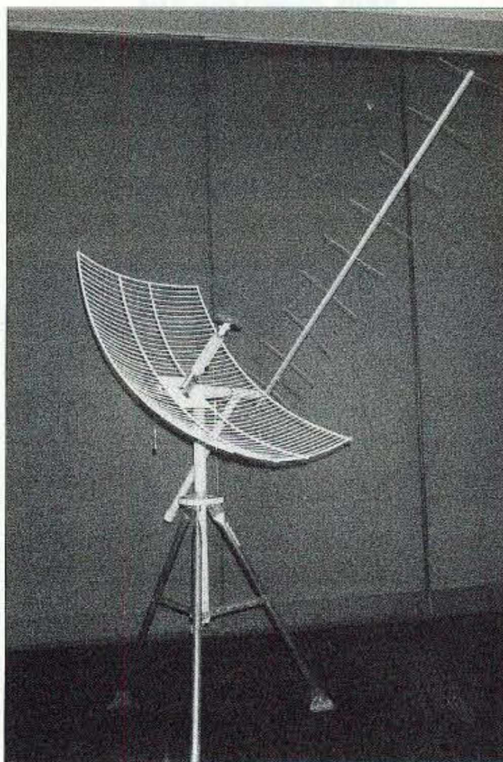
Photo F. A better view of the complete, fully functional AO-40 ground-station antenna system on display and used at Ham-Com 2002 for demonstrations. The system has a linear yagi for the 70-cm uplink and a BBQ-grill semidish with modified commercial downconverter for 13-cm receive.
