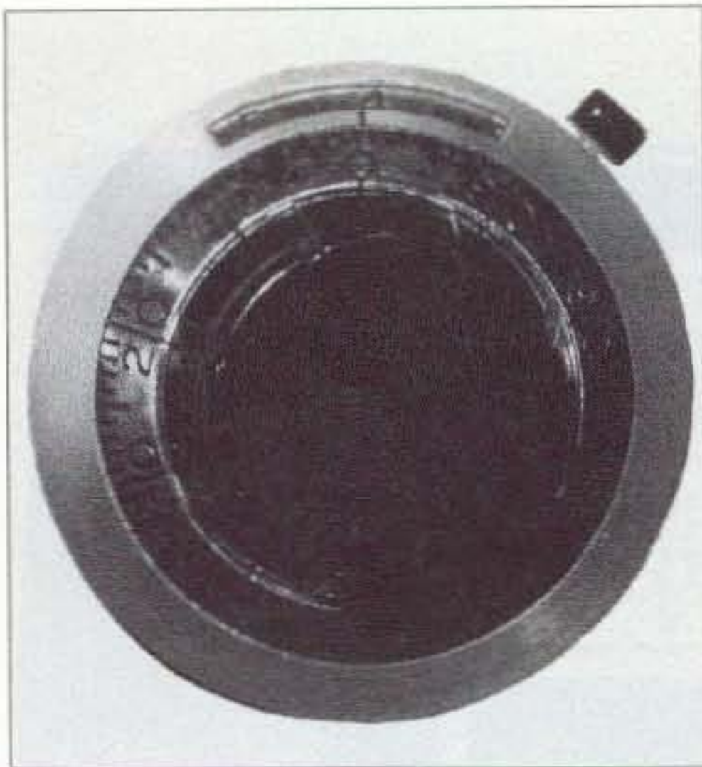
Photo Q. This is a multiturn dial designed to be used with a 10-turn potentiometer.
