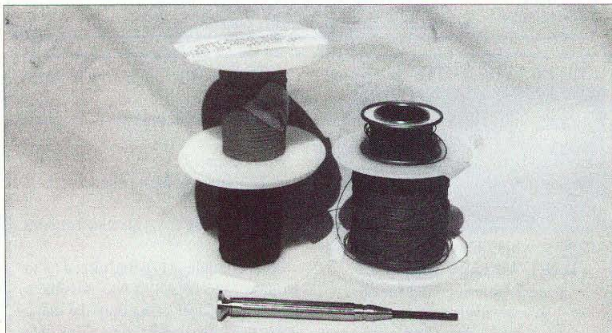
Photo C. A wire-wrap/unwrap tool, with spools of AWG-30 "Kynar" WW wire in the background.
