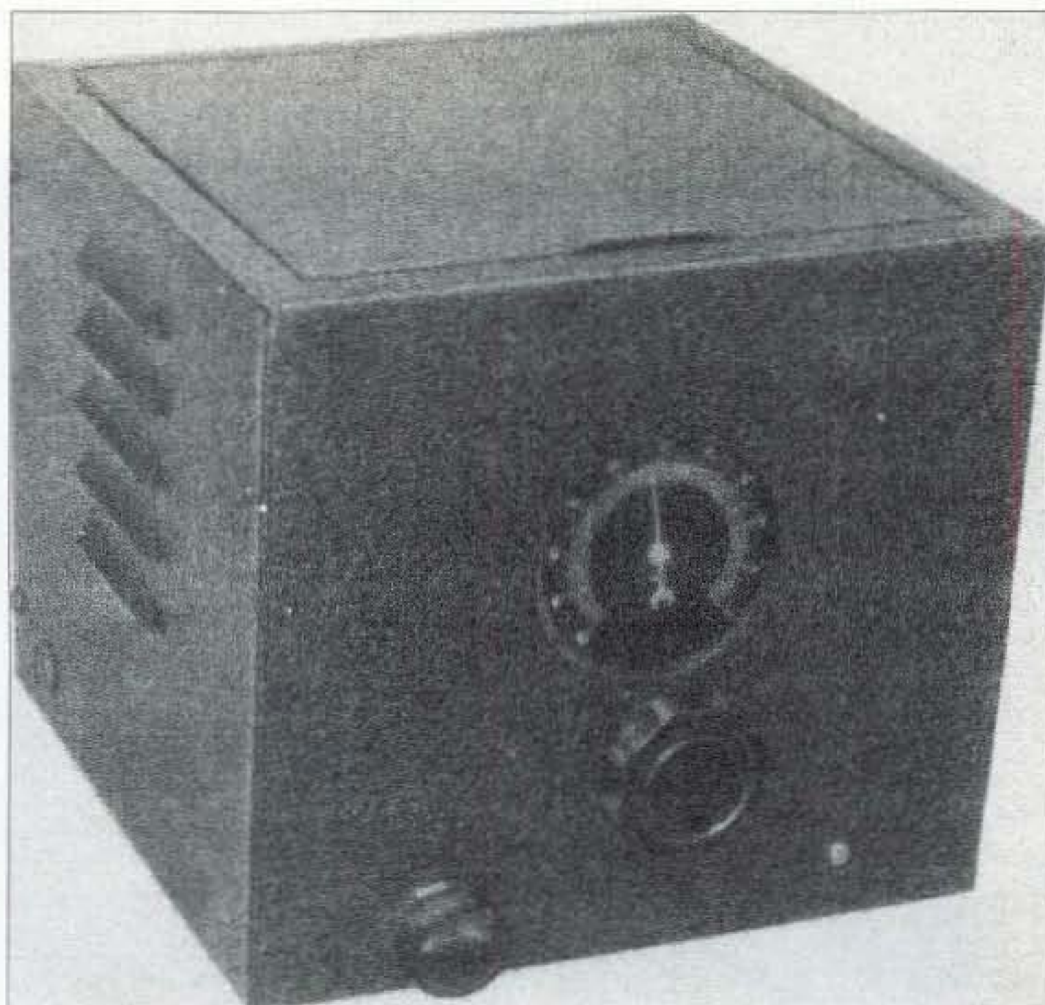
Photo H. This picture shows one of the early uses of a dial cord-driven dial. Some commercial radios of this era used a flat rubber drive belt instead of dial cord. (Photo ref. 3, pg. 150)
